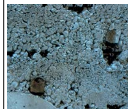
Poor quality concrete – Honeycombing and timber.
